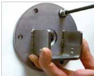
Secure the motor flange using the short M8 bolts with neoprene washers.
