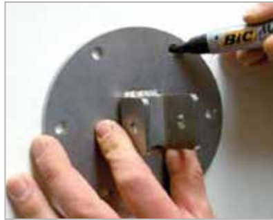
Mark the drill holes for the bearing flange.
