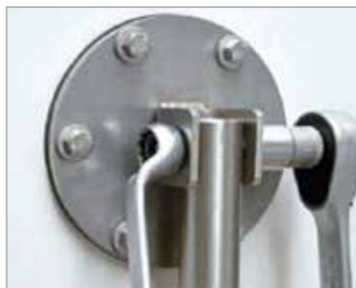
Attach the bearing shaft with bolt and self-locking nut.
