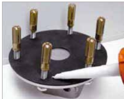
First thread the WAKO plugs onto the bolts (with neoprene washers), then apply sealant to the seal.
