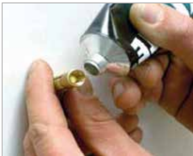
TIP! A bit of grease inside of the WAKO plug prevents the entry of dust that makes the bolts difficult to turn.
