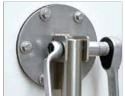
Attach the bearing shaft with bolt and self-locking nut.
