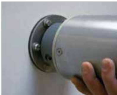
Slide the winding tube over the U-profile. ATTENTION! Continue to feed the cable through so it won't be damaged.
