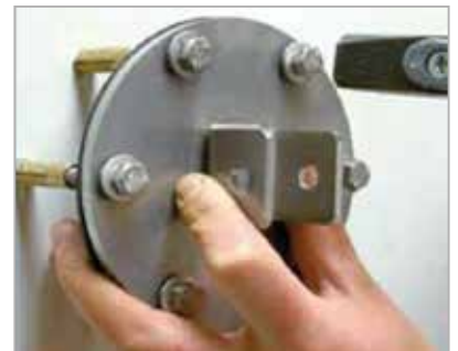
Position the bearing flange and drive in the bolts until they are flush with the flange.
