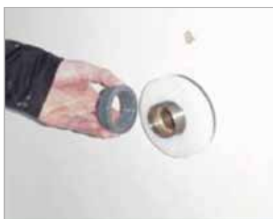
Fit check nut (hand tight).
