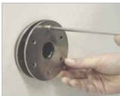
Remove liner flange.
