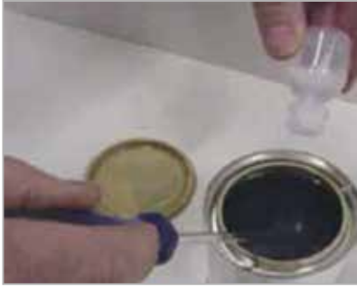
Add hardener to resin and mix well.
