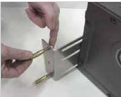
Screw tap bolt + plug together on motor bracket and apply grease in the motor bush.
