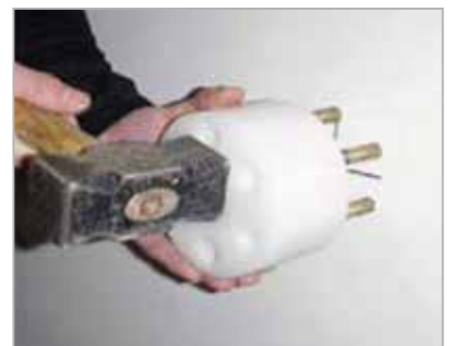
Fit bearing block.
