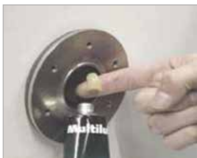
Apply grease in the bronze bushings.
