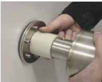
Slide out drive shaft, fit spacer bush in between and secure with M10 bolt.
