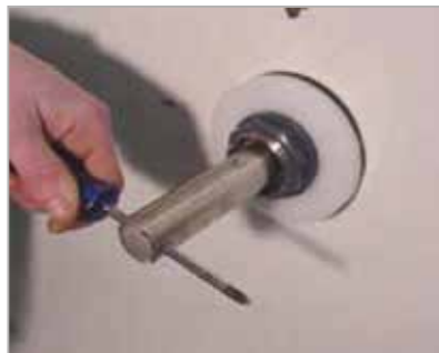
TIP! Use drilled hole at keyway to move shaft.
