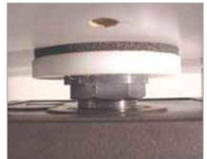
Place motor flush against threaded end to prevent movement of seal and then secure motor bracket on wall side and motor side.
