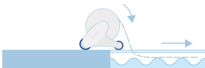
USE THE KEY OPERATED SWITCH TO AUTOMATICALLY ROLL OUT THE COVER ON THE WATER.
