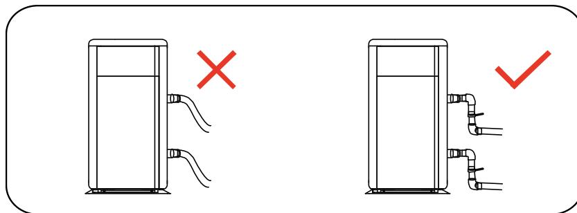
2.1.2. In order to guarantee the heating efficiency, the water pipe length should be  $\leq 10\text{m}$  between the pool and the heat pump.
